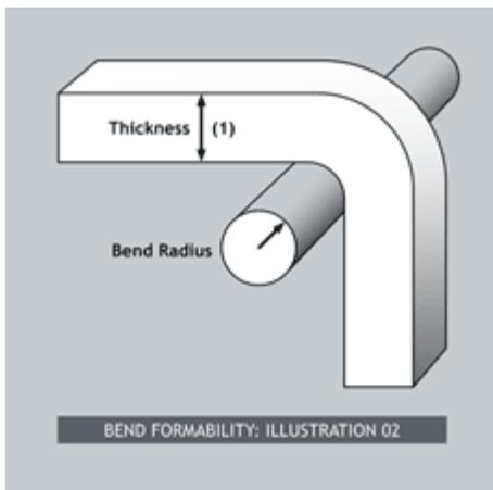
Another factor that allows for better bend formability in wire as compared to strip relates to the width to thickness ratios of the materials. Wire typically has a width to thickness ratio of one (1). Therefore, the deformation mode for wire is plane stress which allows for more formability before fracture.
