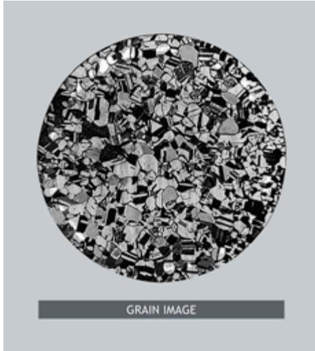
They are composed of aggregations of crystals joined at boundaries. Aggregations of unit crystals are termed Grains and the boundaries between them are the **Grain Boundaries**.
